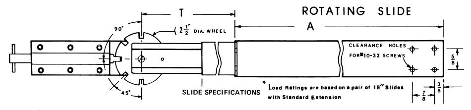
ALL HARDWARE STAINLESS STEEL OR ZINC PLATE FINISH: Molybdenum Disulphide. Dry Lubricant, baked on at 400° per Mil-L-25504 over Phosphate Coating per Mil-P-16232, Type M.
